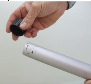
2......Once bung is removed the tubing is visable and the 2 indentations which prevent the inner pole coming out.
