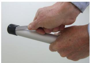
1....To remove bung at bottom of pole, use the handle of a spoon to break any seal to the pole
